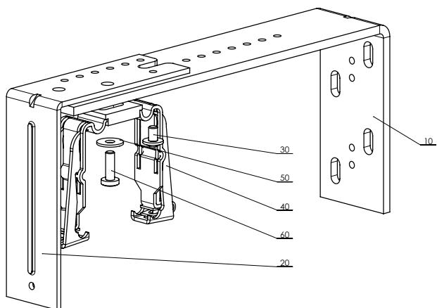
Support reglable double - mecanique 306 – 368 mm
