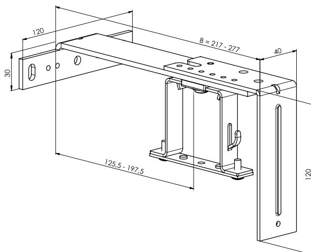
Support reglable - mecanique 206 – 268 mm
