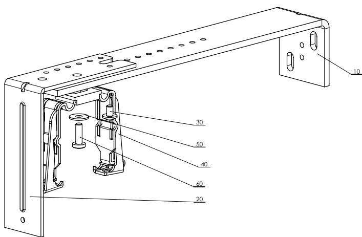
Support reglable double - mecanique 206 – 268 mm
