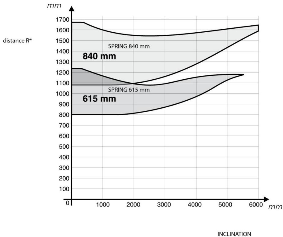
\* READ THE DISTANCE R IN THE COLOUR ZONE DEPENDING ON THE TYPE OF SPRING (650 mm / 850 mm).
