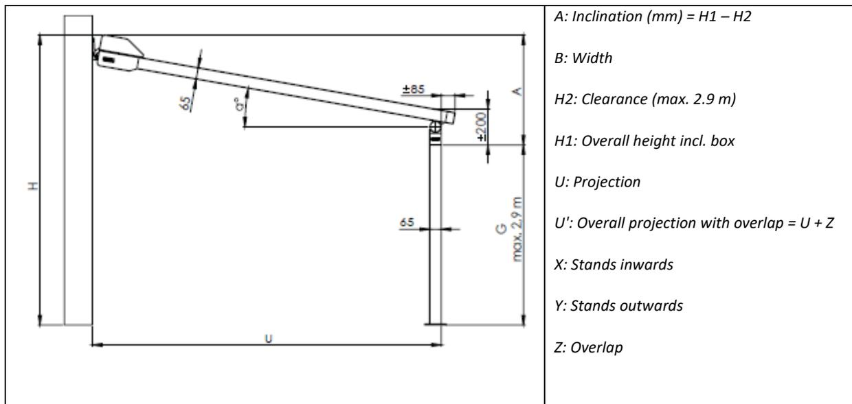
**INCLINATION (A) in MM**
