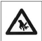
PREVENT THE RISK OF BEING SQUEEZED (LOOSE GARMENTS) NEAR THE CYLINDERS. A RISK OF SHEAR EXISTS WHERE THE EXTENSION POLE PASSES THROUGH THE CYLINDERS. THIS MAY LEAD TO SEIZING AND SQUEEZING.
