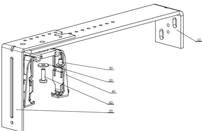
Support reglable double - mecanique 206 – 268 mm
